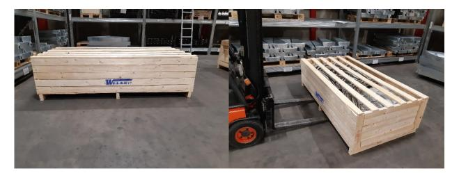
Spiral staircases come packed in a box that is balanced. Lift using a standard forklift rack on a truck or wheel loaded with the forks as far apart as possible.
